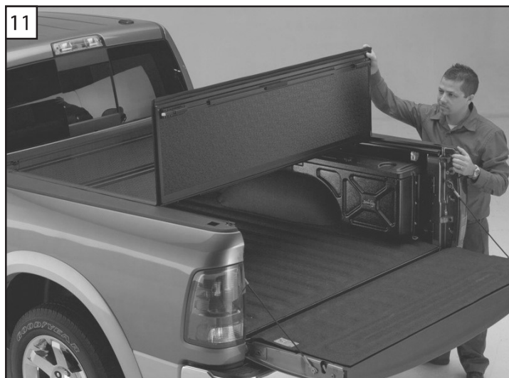
10 & 11. Once the cover is located correctly, fold the cover to the open position. Pull the release cables on the rear panel to release it from the side rail. Take care to fold it gently so the position of the cover is not disturbed.
