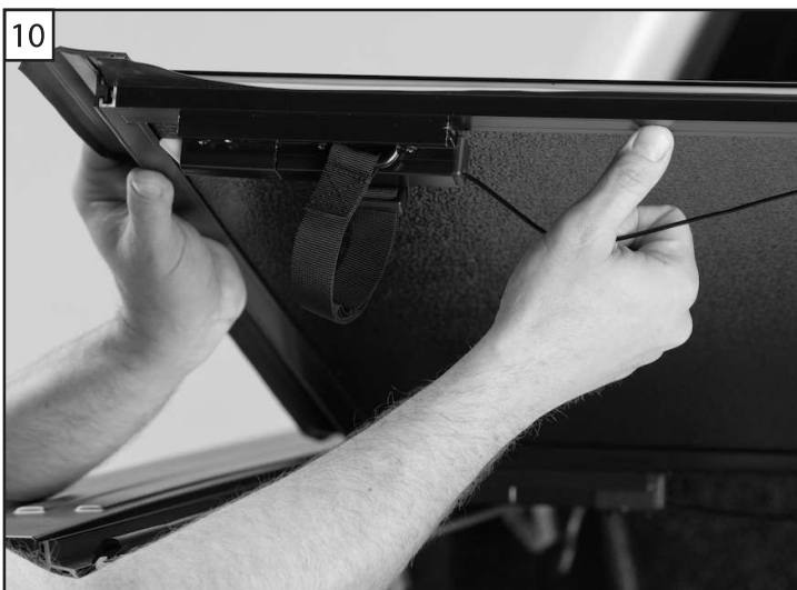
10 & 11. Once the cover is located correctly, fold the cover to the open position. Pull the release cables on the rear panel to release it from the side rail. Take care to fold it gently so the position of the cover is not disturbed.
